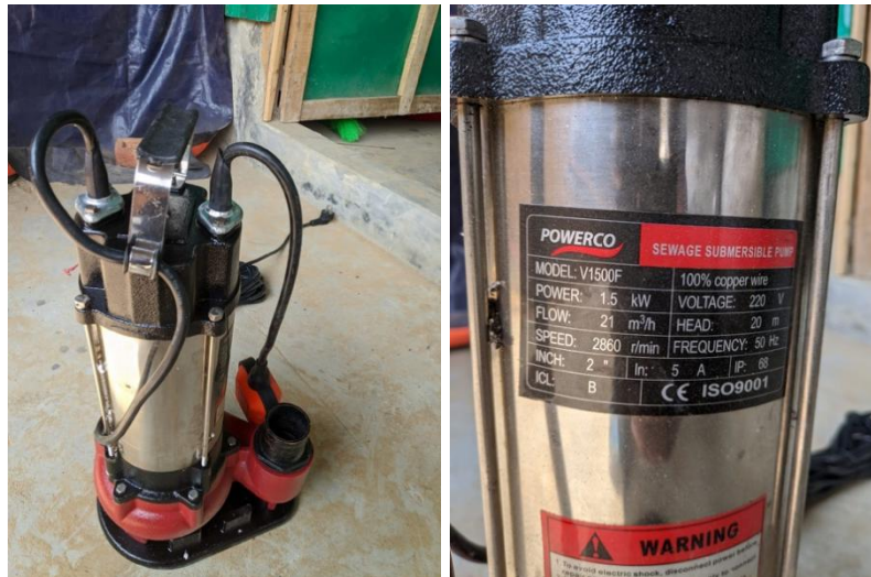
Figure 10: Sludge pump used by BRAC for pumping faecal sludge to transfer stations in Camp 14. (Source: BRAC 2020).
