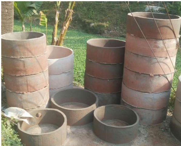
Figure 7: Concrete rings used for pit construction (Source: UPM 2020).
