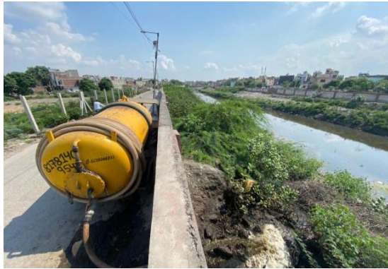
Figure 12: Private desludgers desludging faecal sludge into an open drain (Source: Sachin Sahani/CSE/2021).
