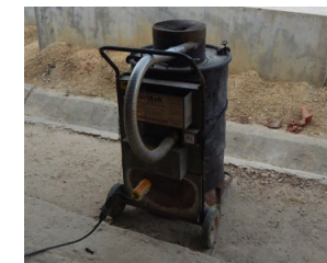
Example of portable incinerator (and ash pit behind).
