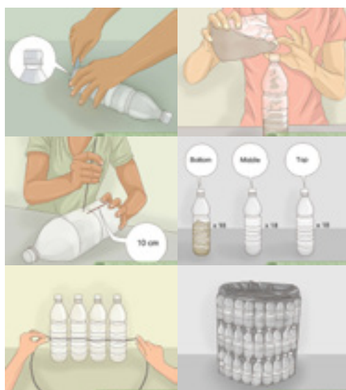
Figure 35: Making a waste bin from plastic bottles (source: Blueschools Kit)
