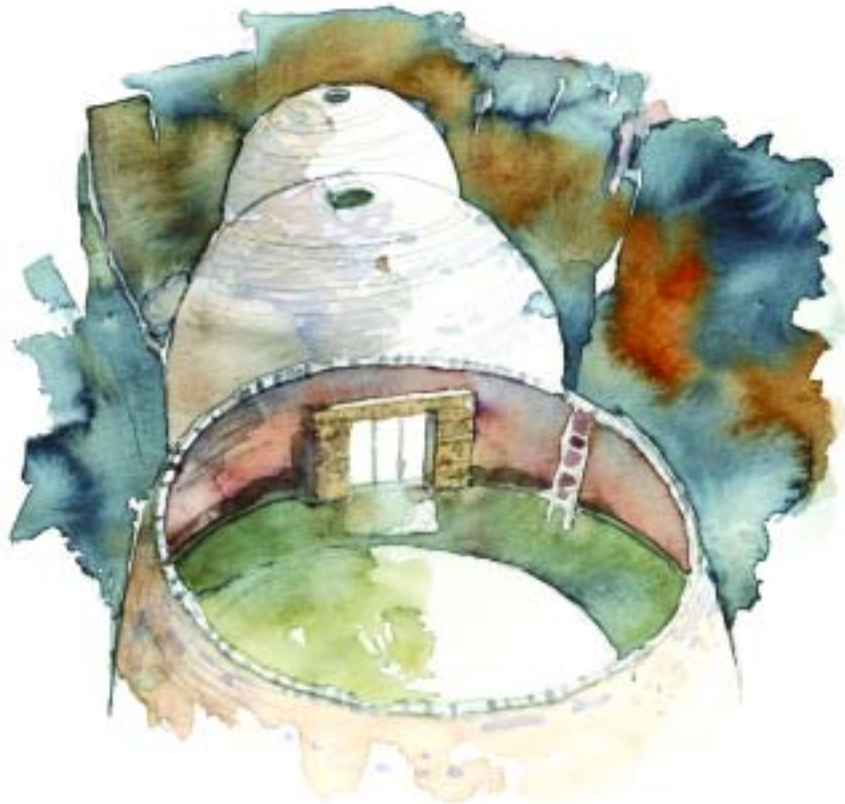
Cross-section of a 100-m 3 biodigester module
