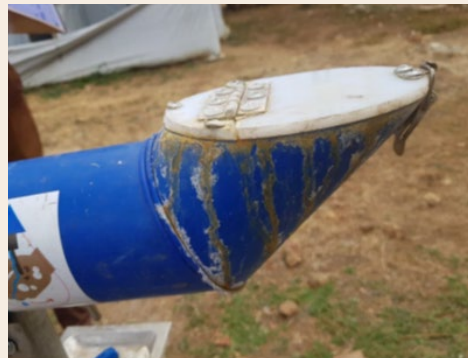
FIGURE 27 // TOP: Cleaning inside of the WASHaLOT with a brush (Source: GIZ Fit for School, photo by David Weyand, 2020) FIGURE 28 // LEFT: Examples of algae proliferation and mineral deposits due to poor maintenance (Source: photo by S. Samiyaga, 2021)
