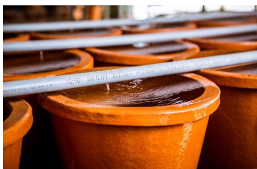
Figure 4: Testing flow rates of the filters
