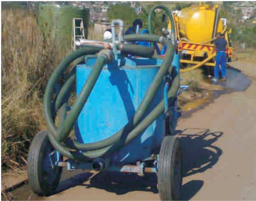
Figure 30 : Vacutug being trialled in Pietermaritzburg
