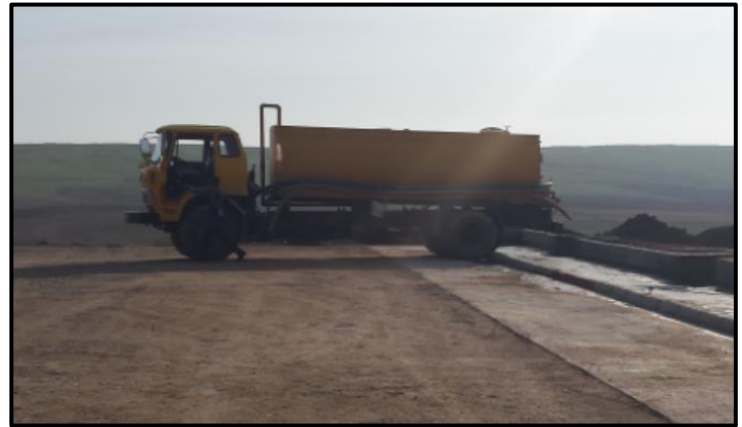
Figure 6 - 10,000l Contractor Vacuum Truck (Source: Author, 2018)
