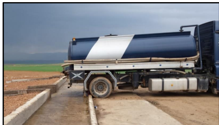
Figure 8 - 10,000l Contractor Vacuum Truck (Source: Author, 2018)
