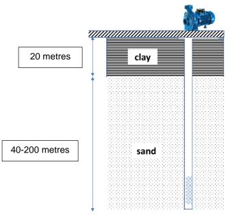
Figure 7: Soil profile in Naogaon district and location of tube well screen.
