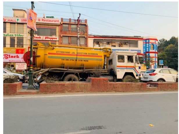
Figure 4: Sewer jetting cum suction machine (Source: Laila/NIUA/2022).
