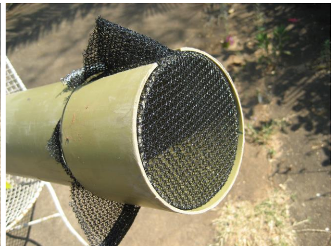
One method of attaching the shade cloth to the pipe
