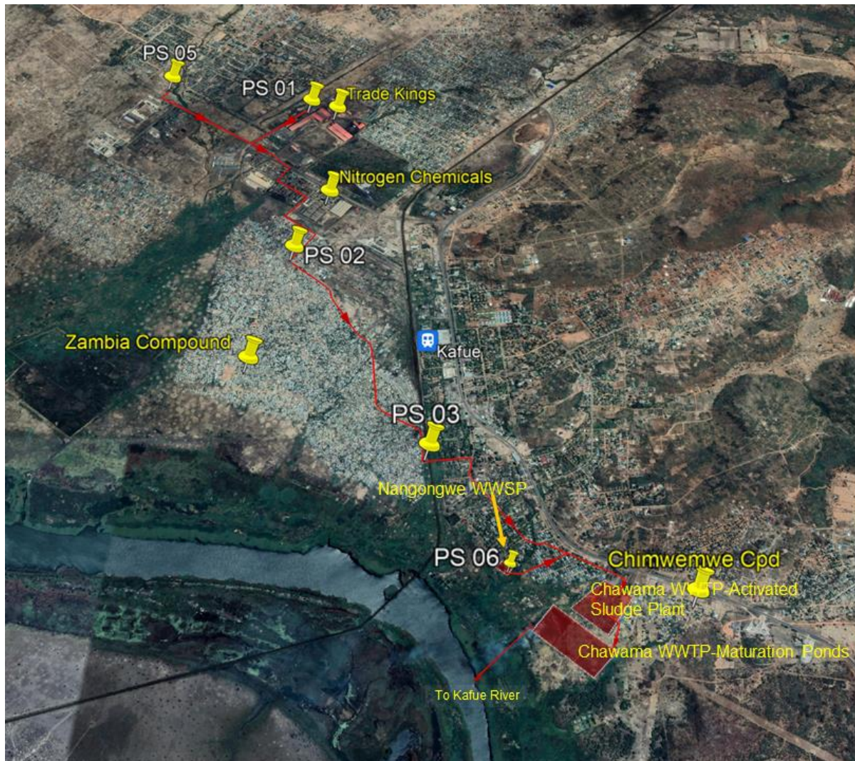
Figure 3: Location of Pumping Stations and Treatment Plants in Kafue (Note that the route for the lines is not known and therefore the presented routes in the Figure are imaginary).
