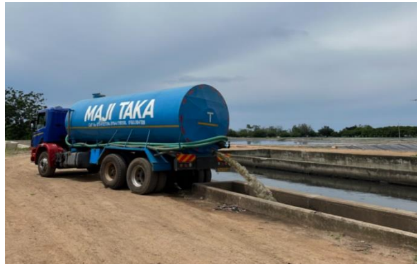
Figure 14: Private Deslugger decanting at the FS decanting point at WSP Butuja. (Source: Harsh/CSE/2022).
