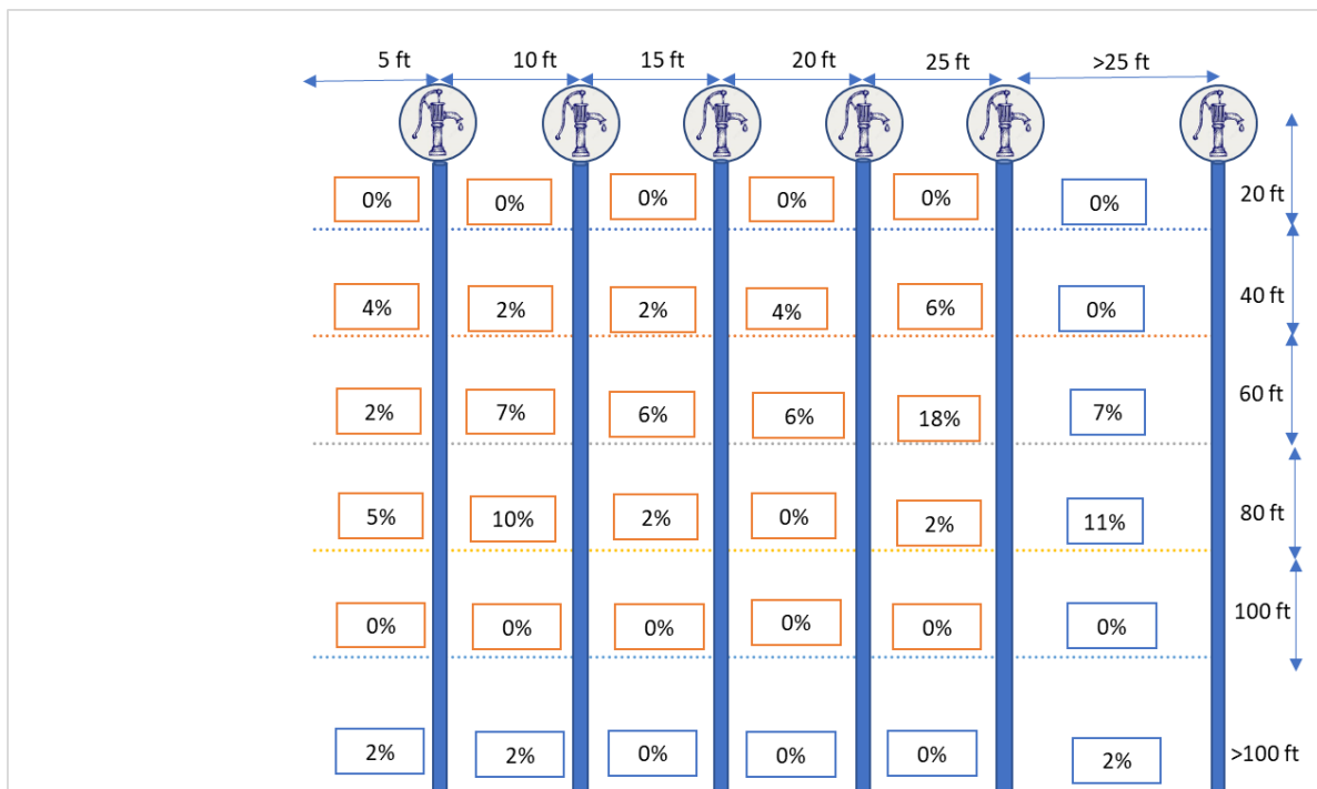
Figure 11: Depth of hand pumps and wells and lateral spacing of it with containment types lined pit with semi-permeable walls and open bottom.
