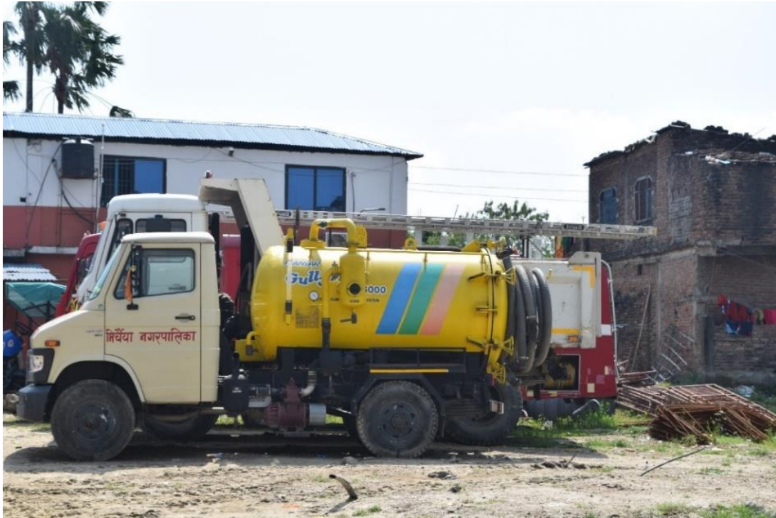
Figure 13: Desludging vehicle of the Mirchaiya Municipality.
