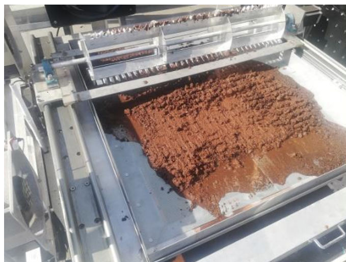
Figure 3.9. Wet soil tests setup with rake system in operation
