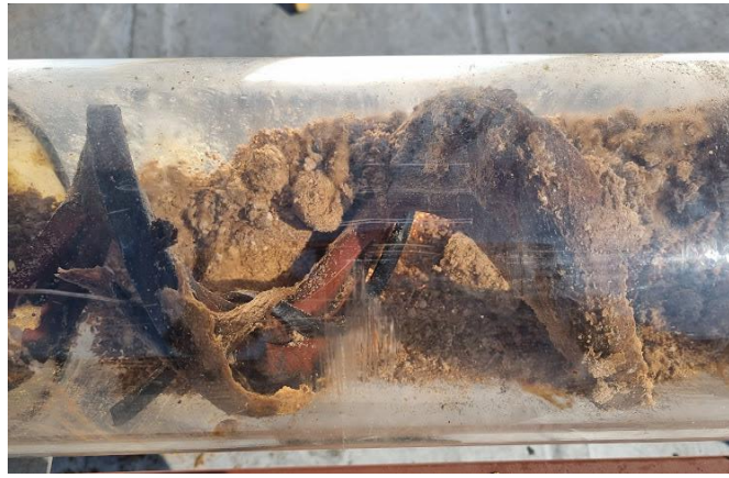
Figure 4.27. Drying of the 50% moisture content sludge
