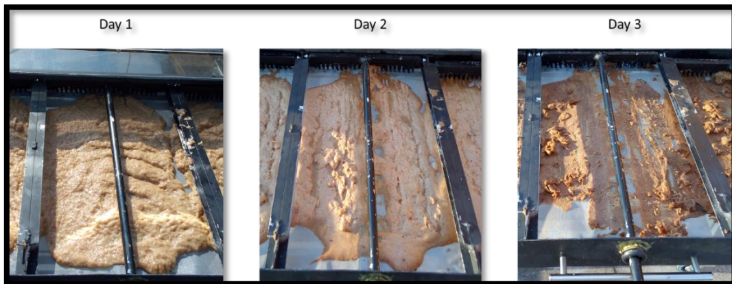
Figure 2.2. Photographs of the faecal sludge simulant inside the solar dryer at different days of experiment
