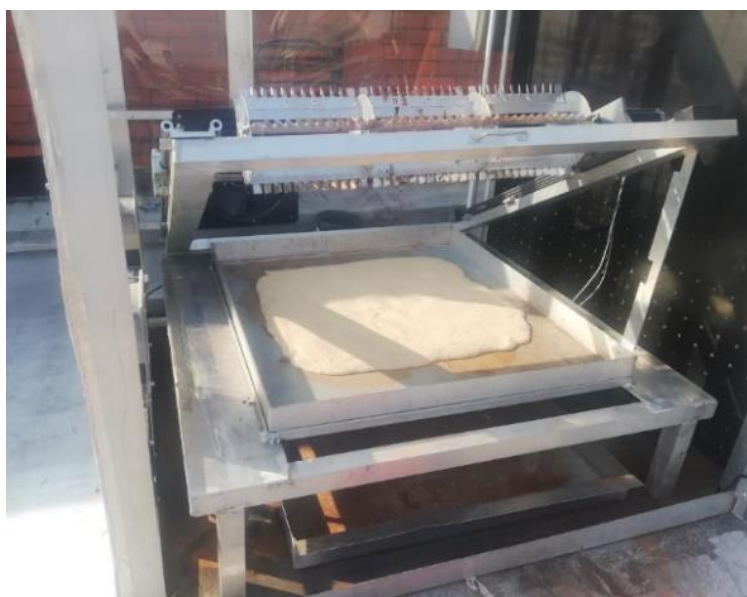
Figure 3.10. Synthetic sludge tests setup
