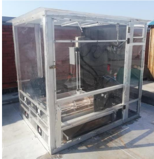
Figure 3.1. Greenhouse Solar Thermal Dryer
