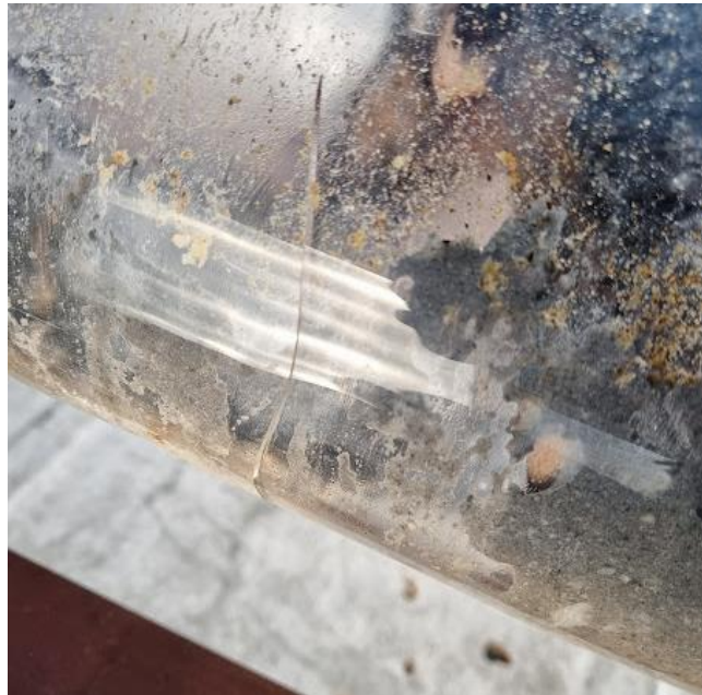
Figure 4.30. Cracked acrylic tube
