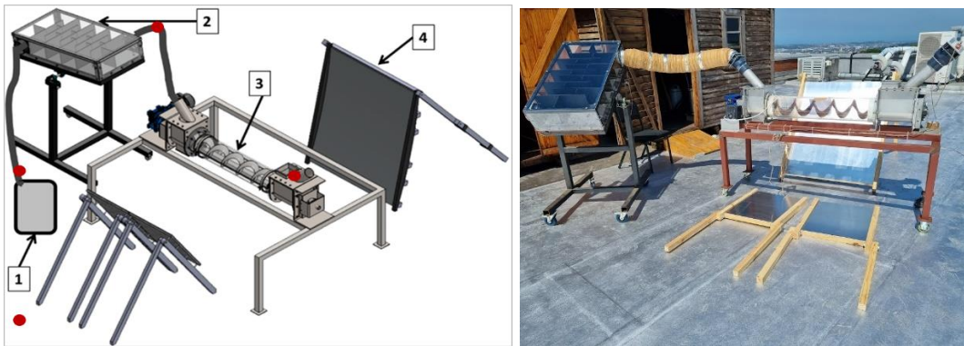
Figure 5.3. Screw conveyor solar drier schematic representation (at the left) and photograph (at the right) {1: air dehumidifier; 2: SAH; 3: DC; 4: reflector; red points: temperature / relative humidity sensors}
