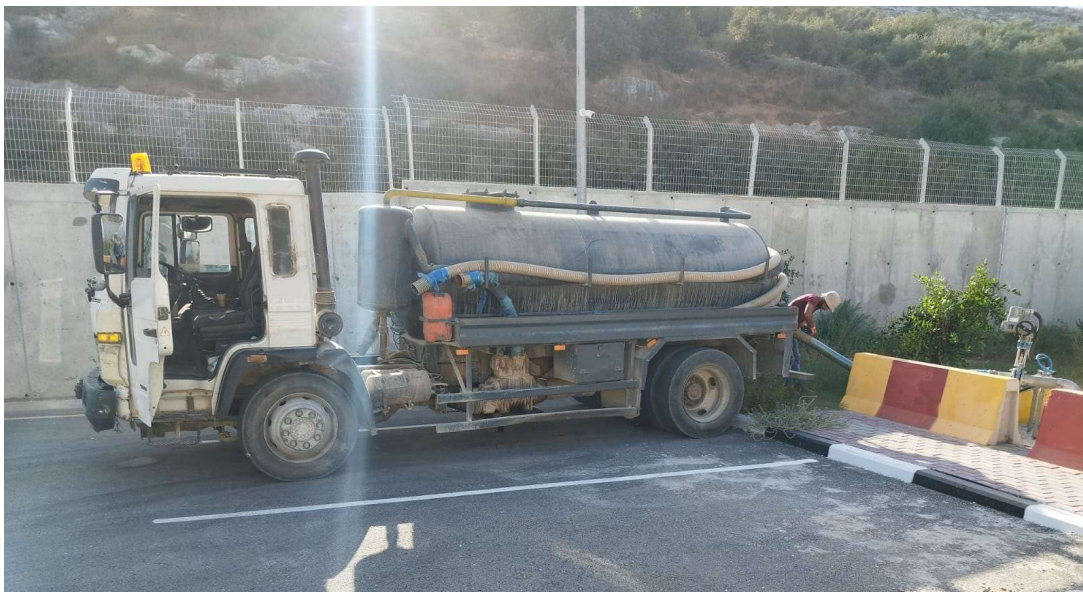
Figure 5: Vacuum truck discharging the faecal sludge at the WWTP of Salfeet.
