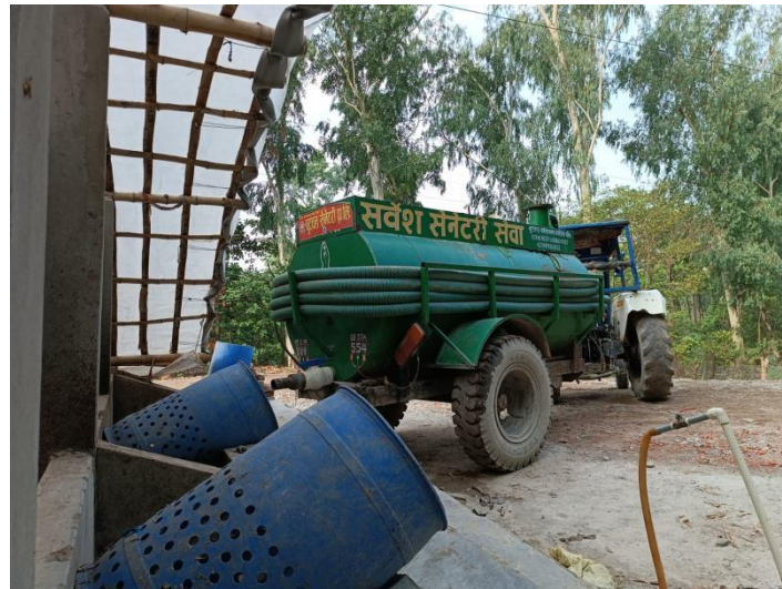
Figure 11: Faecal sludge desludging service provider transporting the emptying faecal sludge to the treatment plant.
