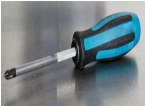
Screw driver (used to tighten screws, nuts and bolts)
