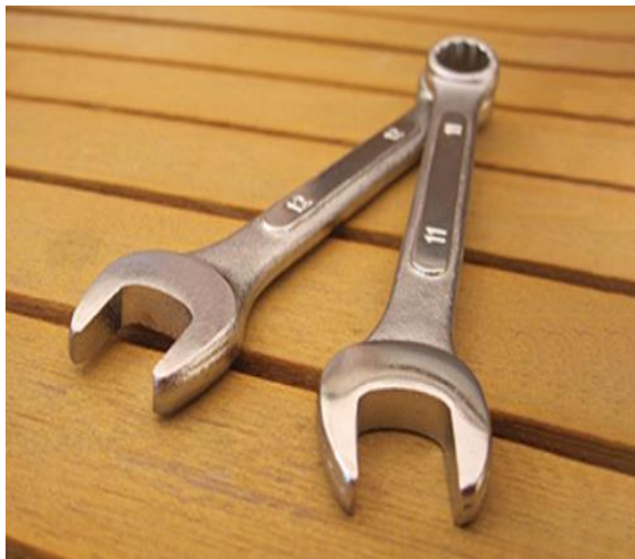
Spanner (used to grip and turn objects especially during plumbing works)
