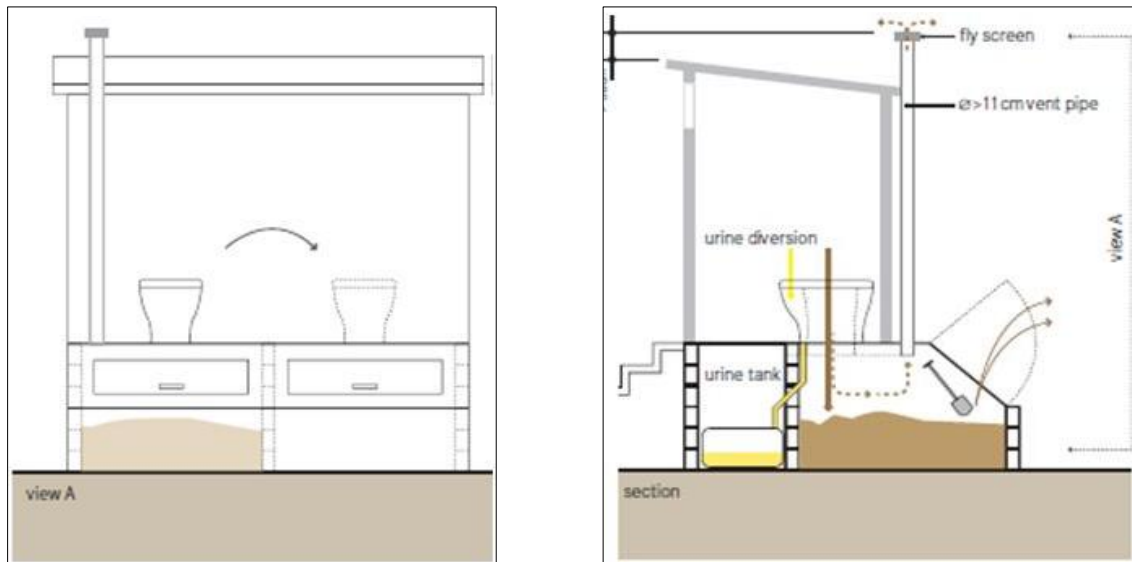
Figure 2 - 3: A schematic of two side views of a double vault UDDT showing the two faecal collection chambers and separate urine collection (source: Tilley et al., 2008). (Diversion of anal cleansing water is not shown here).
