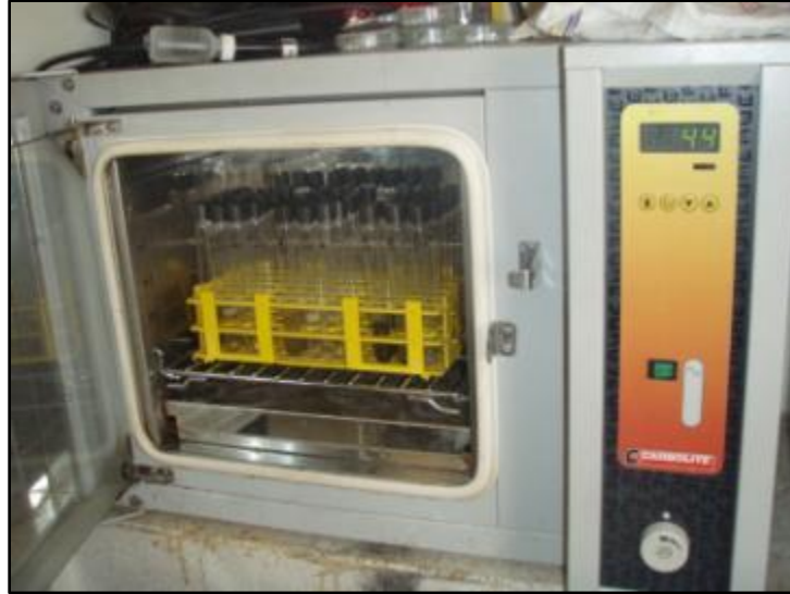
Figure 4: Incubator with test tubes
