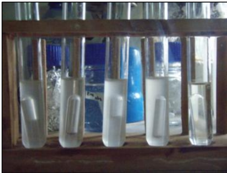
Figure 5: After incubation at 44°C for 24 h, four of the five tubes show gas production
