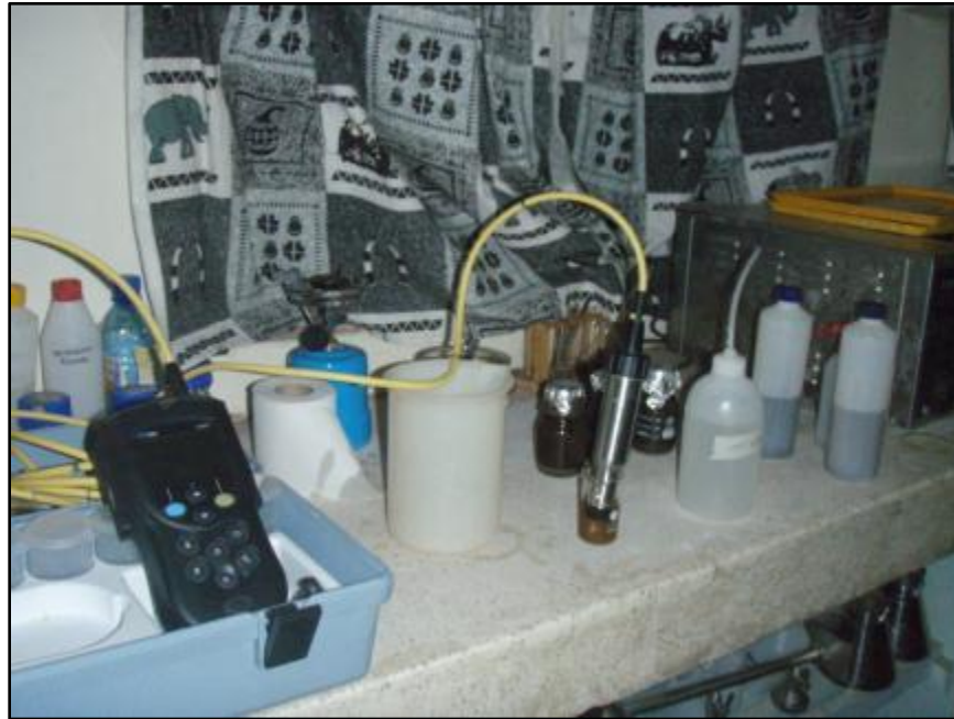
Figure 8: pH meter for measuring pH in urine sample
