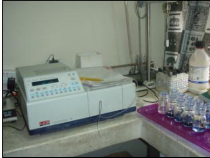
Figure 10: Spectrophotometer for nutrient determination
