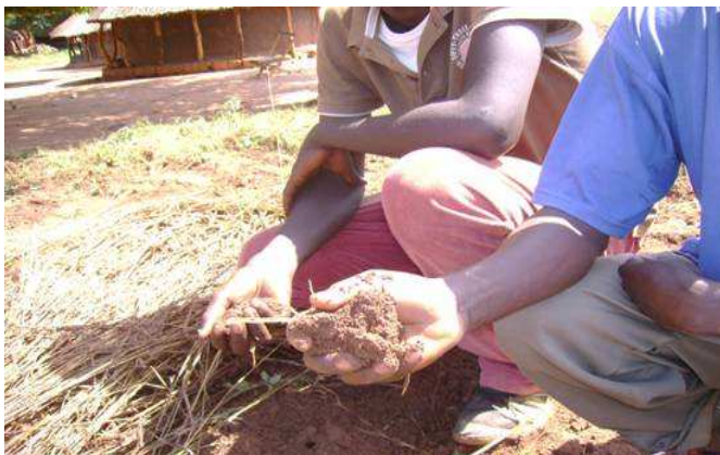
Fig. 5: Estimation of initial moisture level of a mixture of compost and soil by the "squeezing" method (photo by Richard Komakech, 2009).
