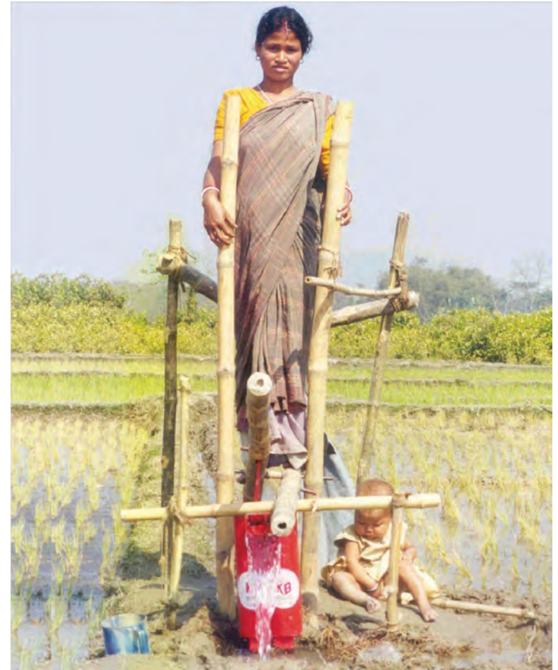
Figure 16. A low-cost pump with bamboo treadle that can be used for furrow irrigation or to fill the tank for drip irrigation.
