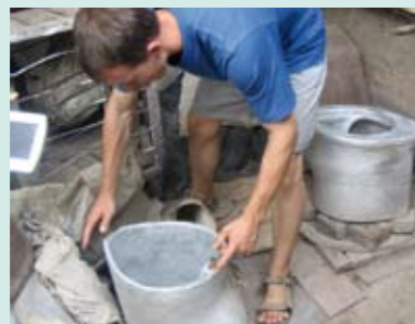
Urine diverting seat riser made from concrete.
