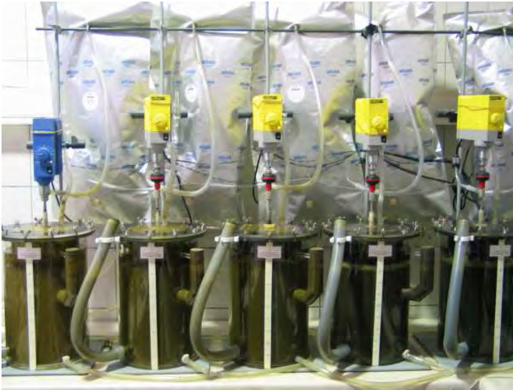
Figure 2: Continuous-flow digestion installation consisting of 10 l double-wall containers equipped with gas bags and stirrers
