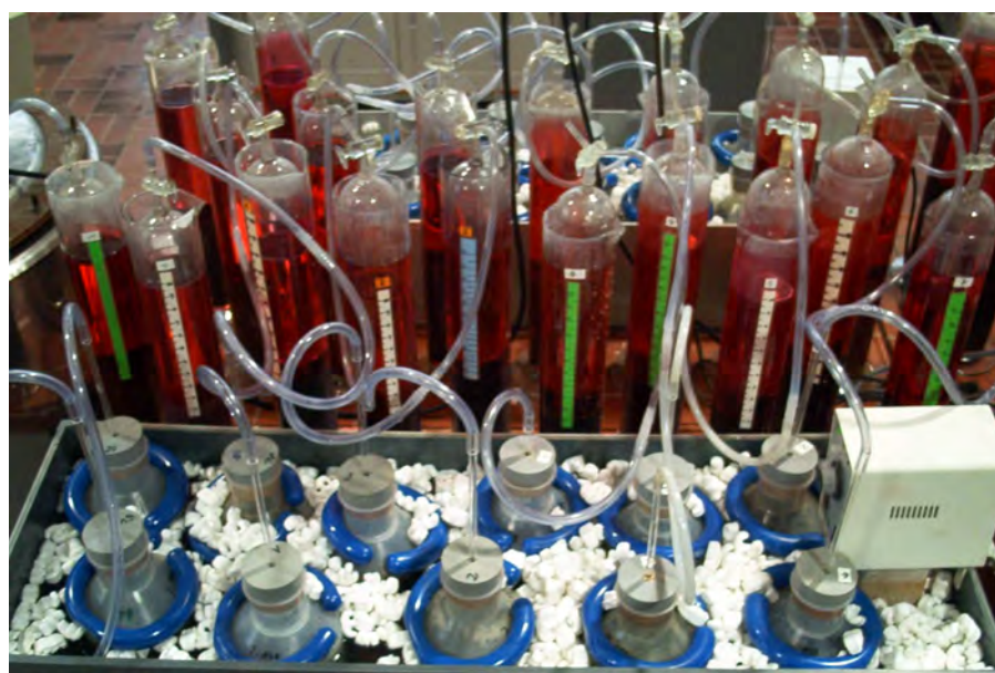
Figure 1: batch digestion test apparatus: in front polyethylene bottles in a water bath, in the rear gas meters with red-coloured water as obstructing liquid
