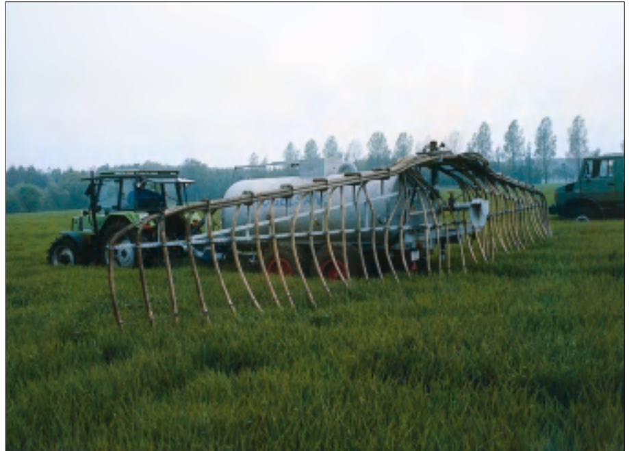
Tank wagon with an applicator fitted with trailing hoses. The fertilizer is usually fed to the hoses through a centrally located distributor.
