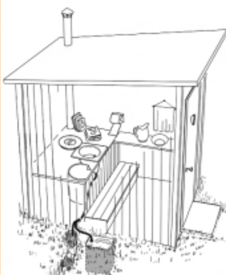
Urine-separating inset for dry closets.
