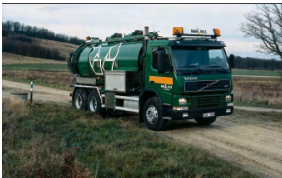
Urine can be transported as far as 220 km by tank truck and trailer before energy consumption exceeds that in the conventional system.
