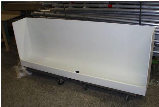
**Fig. 6:** A urinal trough (2 m width) before installation, made of marble powder (source: P. Grönwall, 2006). The outlet in the middle has a Keramag flat rubber tube for odour control, see photo below.
