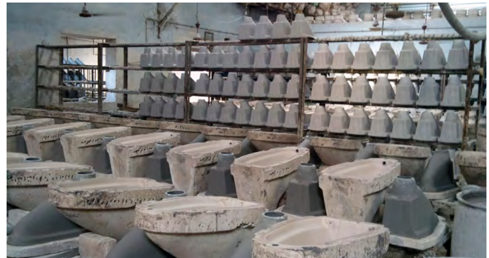
FIG 29. (4.6. DOCUMENTATION OF RESEARCH PROTOTYPING FACILITIES FINDINGS.) Ceramic prototyping tools. Above: tools used for creating ceramics moulds. Below: White painted ceramic ecosan toilets, at Shital Ceramics, Ahmedabad, India.
