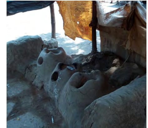
FIG 32. (4.6. DOCUMENTATION OF RESEARCH PROTOTYPING FACILITIES FINDINGS.) Materials and crafts available in the slum. This is a well seen oven in slums in Bangladesh that the team has visited. The clay oven is made of local clay by women living in the slum. On the right picture ovens for sale.
