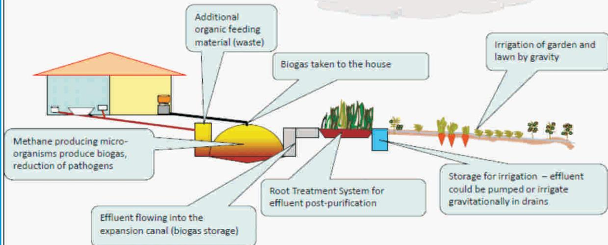
**Sketch of biogas tank.** Wastewater as well as kitchen and garden waste enter the digester and are broken down to biogas and fertile water.
