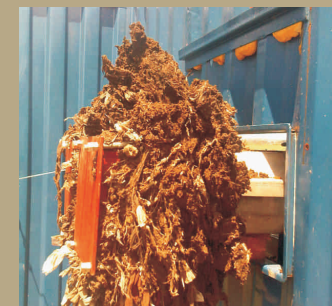
Fig 18. a,b: Semi-dried sludge being loaded into the machine © EWS.
