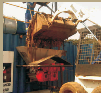
Fig 18. a,b: Semi-dried sludge being loaded into the machine © EWS.
