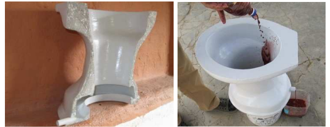
Fig. 4: Cross section of the new urine diversion bowl (left) made from painted concrete where urine collects in the little trough at the bottom as demonstrated in urine diversion bowl (right) (source: CHP, 2009a).
