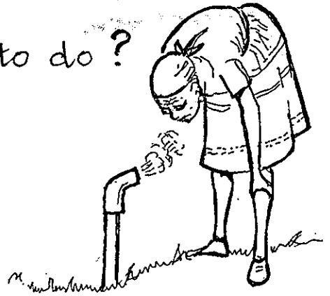
Gas escape through the water trap, which has blown empty. You can smell the gas when you come close to it.
