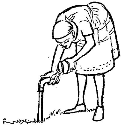
Pour water in the opening of the water trap till it overflow, but not more than one litre.
