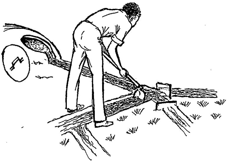
Slurry flows out of your Biogas plant mainly during night hours. Therefore prepare the slurry canals in the afternoon hours.
