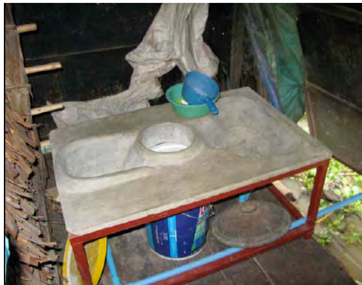
Figure 2: A prototype of a floating toilet (photo courtesy of Michael Brown, et.al)
