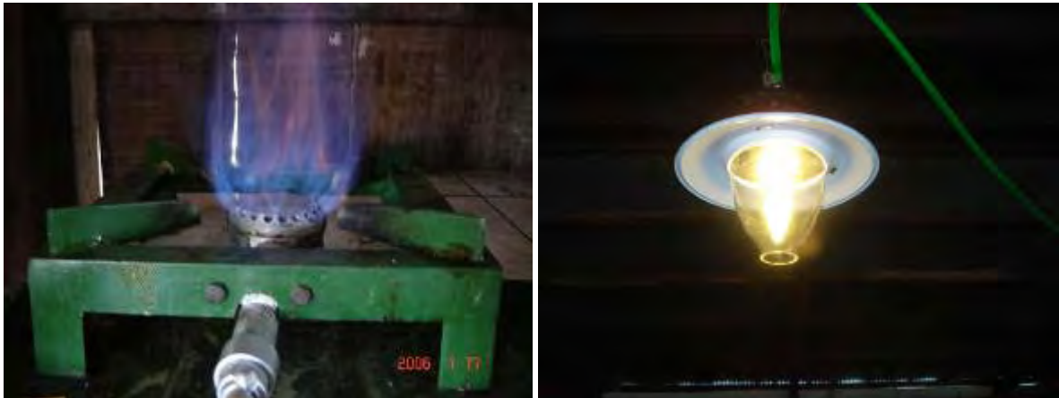
Figure 6. The locally-produced biogas stove (left) and biogas lamp (right), made by DTW
