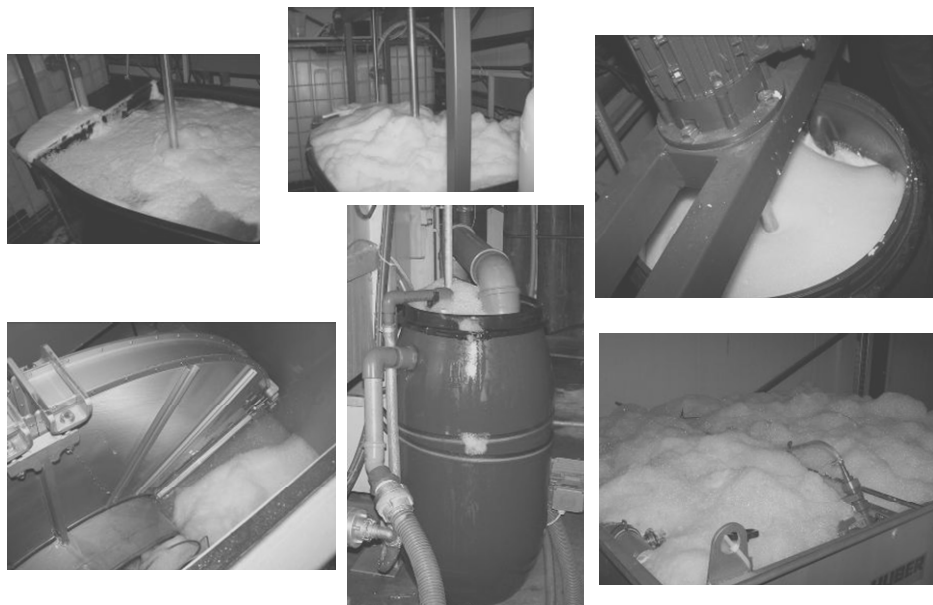
Figure 3: over-foaming by test running in pilot plant in Darmstadt-Eberstadt
