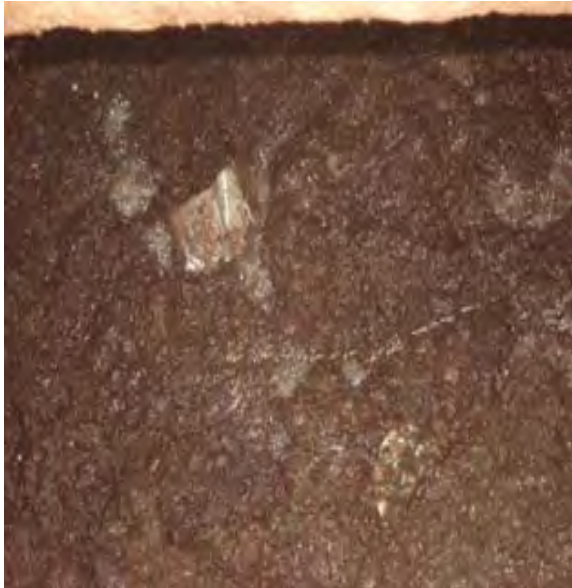
Scum formation in the digesters at Cyangugu Prison
