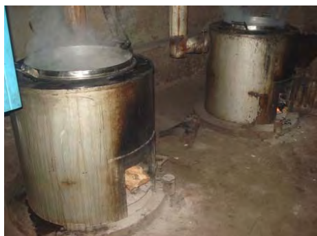
A gas stove transformed into a fuel wood stove because the gas is not sufficient to operate the stove at APENA School
