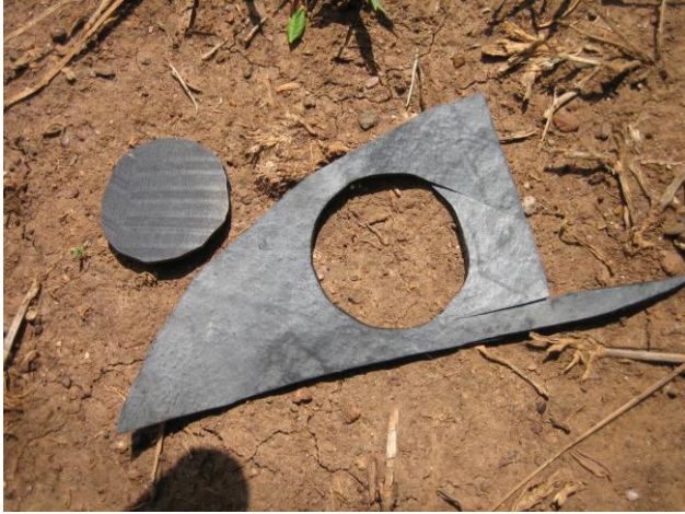
A disc of rubber is cut from an old car inner tube and pushed into the cap to make a better seal
