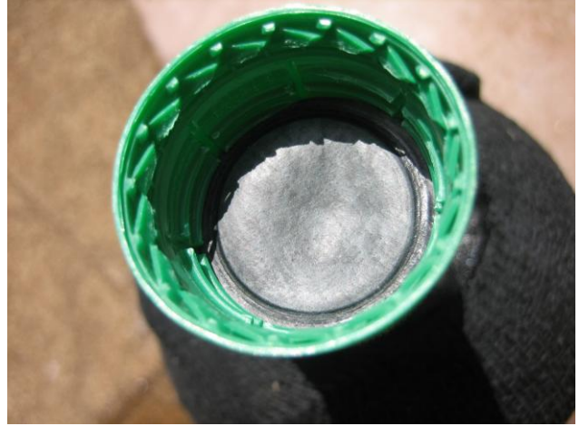
A disc of rubber is cut from an old car inner tube and pushed into the cap to make a better seal
