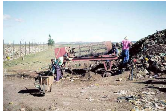
Figure 7 Sieving of matured compost in a rotary sieve at the Rini/Grahamstown (South Africa) co-composting works
