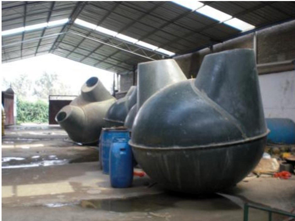
Fibre reinforced plastic digester
