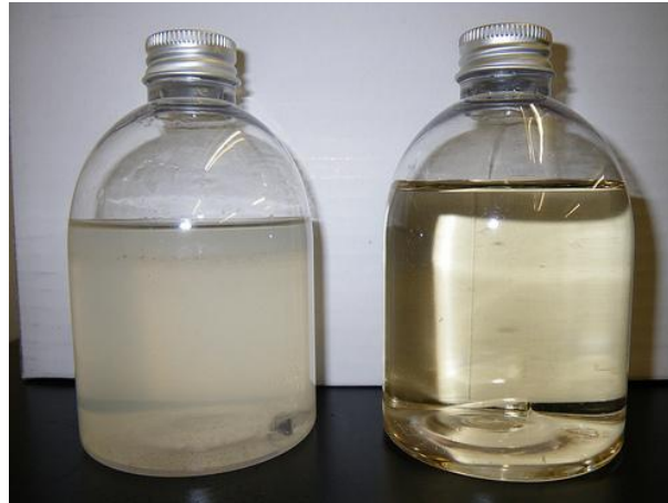
Figure 19: Raw greywater (left bottle), purified greywater (permeate) after treatment (right bottle); (picture by K. Löw)
