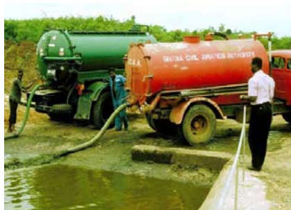
Figure 59. Discharging faecal sludge into WSPs
