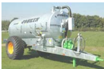
Figure 42. Trailer mounted storage tank
