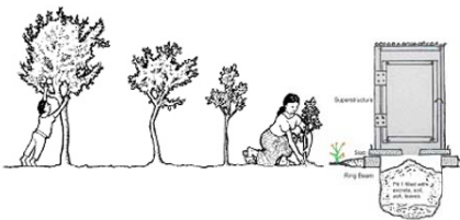
Figure 23. The Arborloo principle
