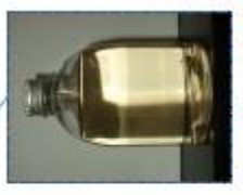
6 - Permeate 280 l/Tag / CSB < 30 mg/l
