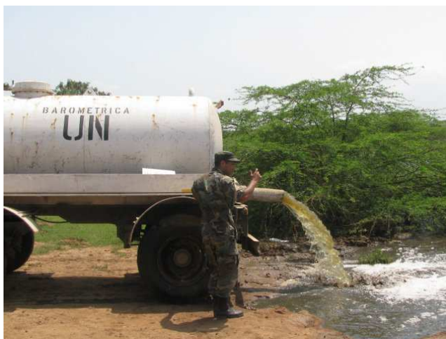
Figure 3: Dumping of sewage or faecal sludge from a UN camp into a lake in the surroundings of Port au Prince in Haiti in 2010 (source: L. Pierre, "Organizing for Haiti", 2010).
