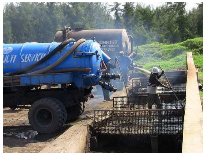
Figure 4: Faecal sludge being discharged from trucks into treatment beds in Cotonou, Benin (source: S. Blume, 2010).
