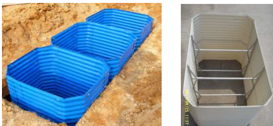
Figure 7: Emergency pit lining kits to avoid collapse. A man hole provides access for desludging. Left: modular corrugated plastic. Right: new design with internal props (instead of relying on locally available wooden props included in former design (source: J. Rhode, Evenproducts, 2011).
