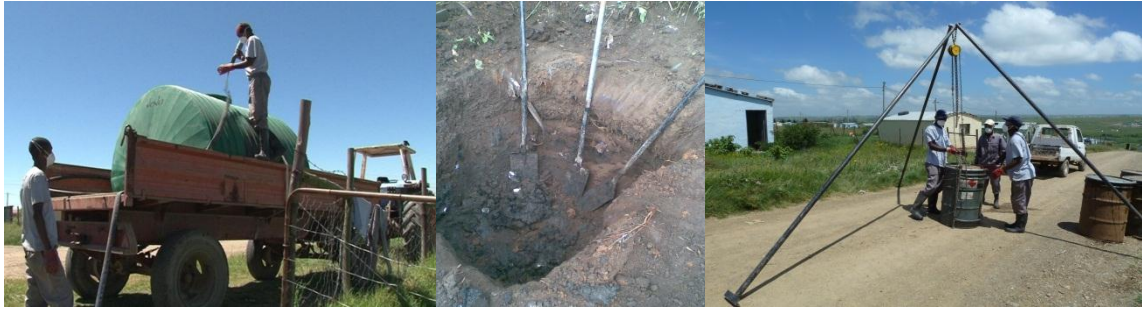
Figure 4 some of the specially designed tools used by franchisees; a tractor mounted tank; long handled spades; drum lifting gantry
