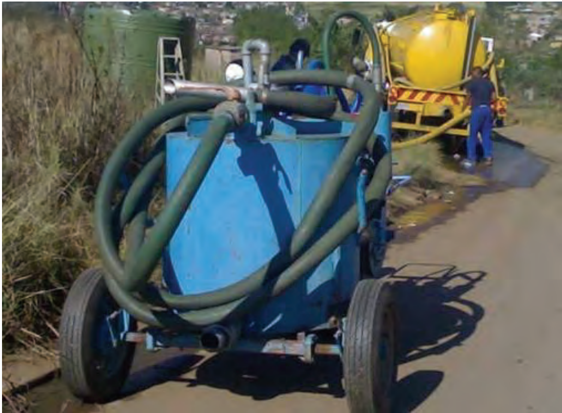
The Vacutug (blue) transferred sludge from the pits of low flush systems in Slangspruit to a 5 m 3 holding tank (green) which was later emptied by a municipal vacuum tanker (yellow).
