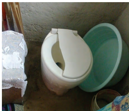
Figure 4.28 Household 14: Householder stood on lid during first week of use and broke it.
