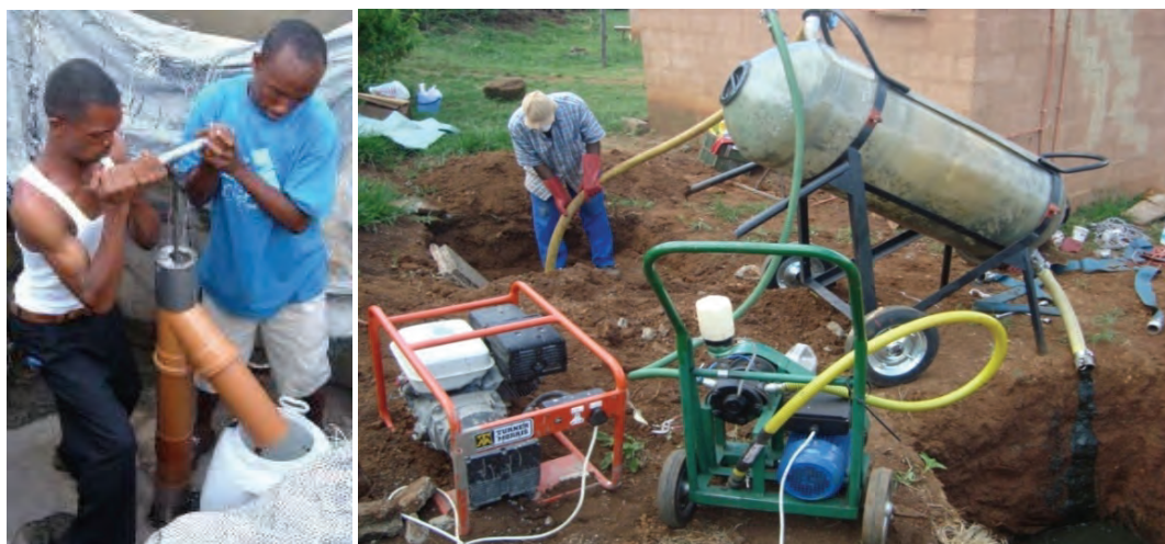
The Gulper (left) a hand operated vacuum pump (Sugden, 2008) and the E Vac (right) and electrically powered vacuum pump developed by Partners in Development
