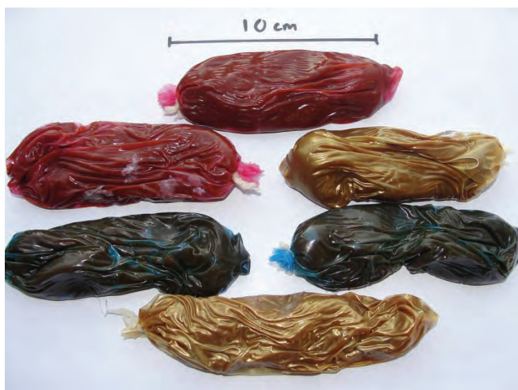
Figure 4.3 The test samples made up according to the method prescribed by the MaP test protocol. Each sample contains 50 grams of soy paste, and is contained in a latex sheath.
