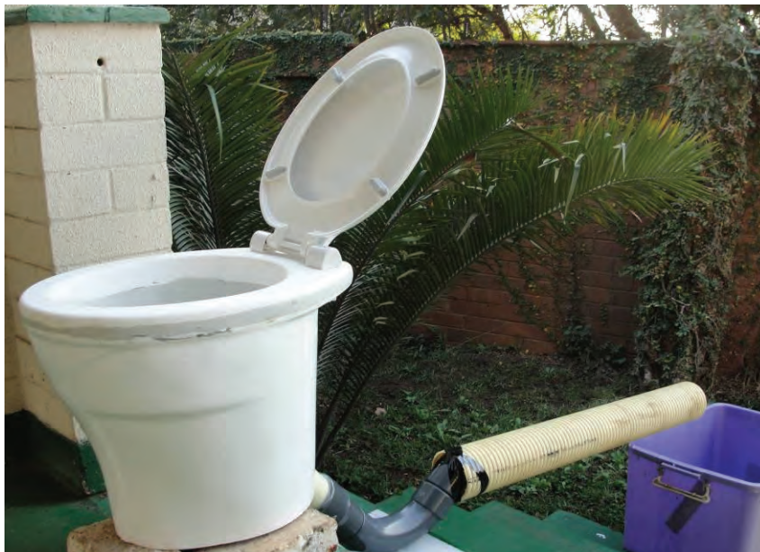
Figure 4.4 The test set-up. For each flush test up to six 50 g replica faecal samples were placed in the pan with a prescribed amount of toilet paper (20 squares of single ply).
