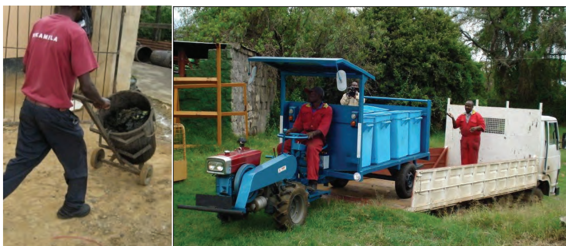
Drumbarrow used by eThekweni (left) and Chinese two-wheeled tractor with trailer transporting bins to truck for road transport (right, UN HABITAT 2009)
