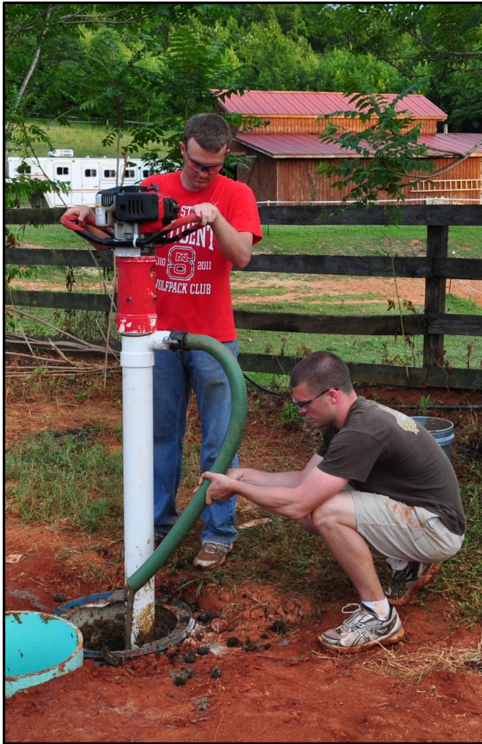
Pit Latrine Extraction Auger lifting simulant waste from a 5 foot deep pit.
