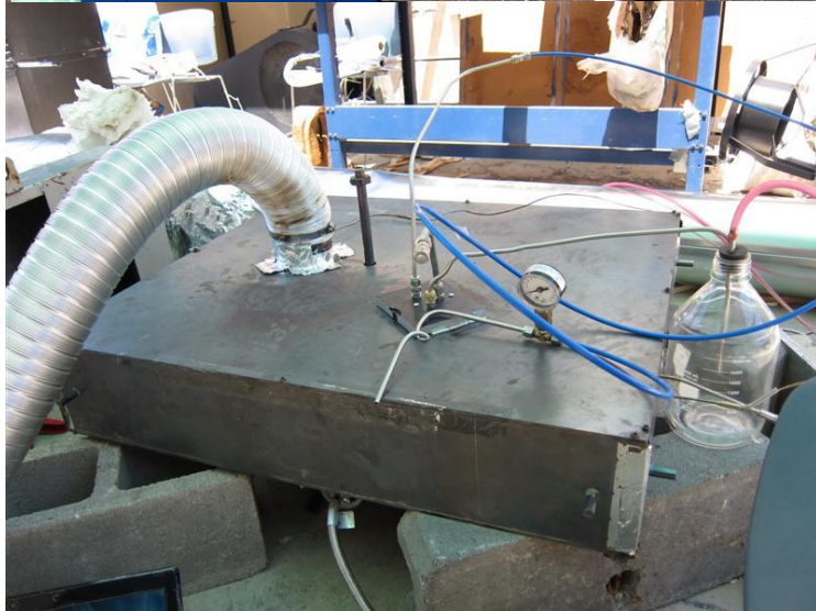
Conversion of solid waste into biochar using pyrolysis at community-scale facility
