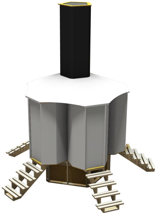
5-toilet array with composting structure below and ventilation plenum above
