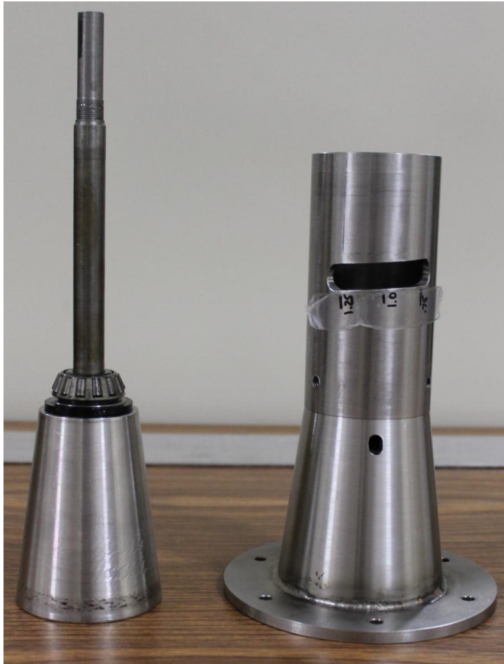
Fecal treatment chamber housing (inverted). The 10 cm, tapered section is the reactor rotating core (left) and the shell (right).
