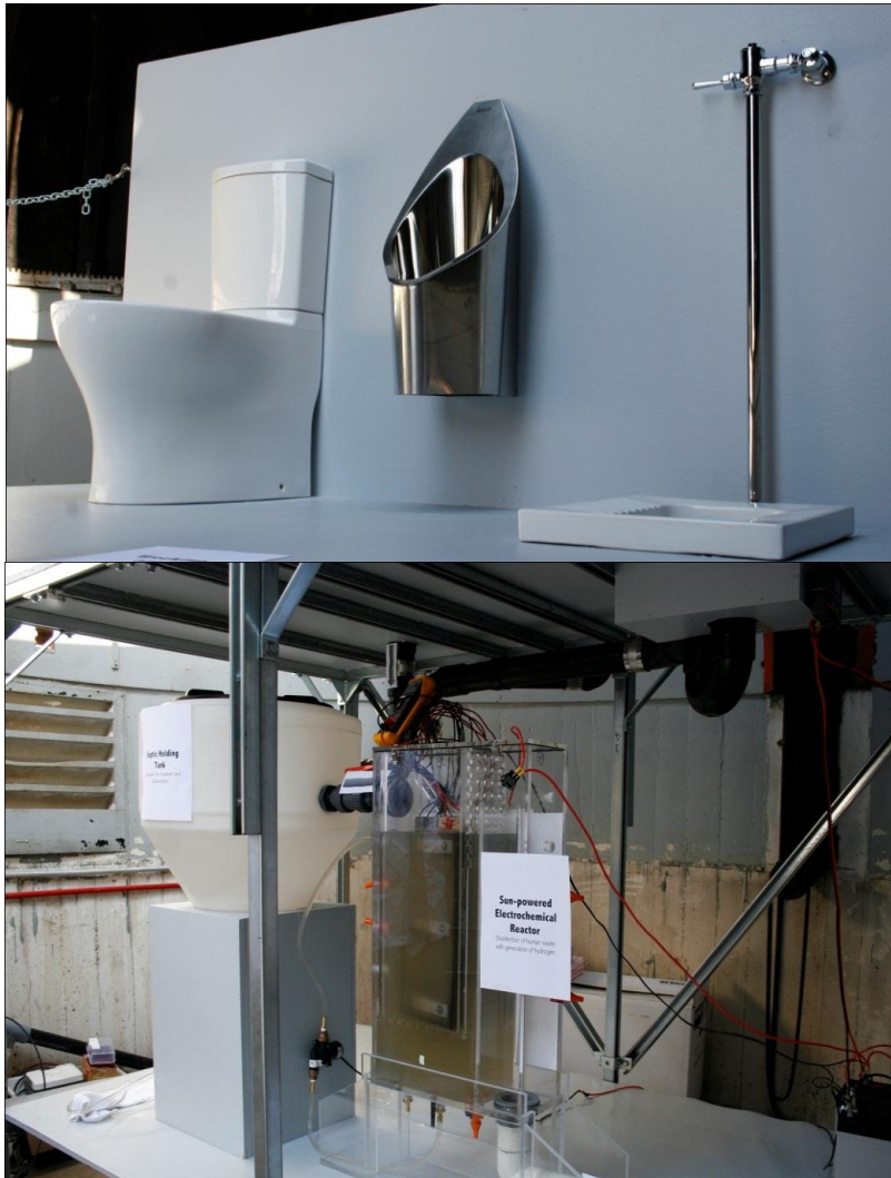
The Caltech RTTC Solar Toilet First-Phase Demonstration System
