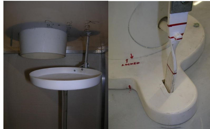
Washwater diversion and odour seal mechanism on three-way split pedestal
