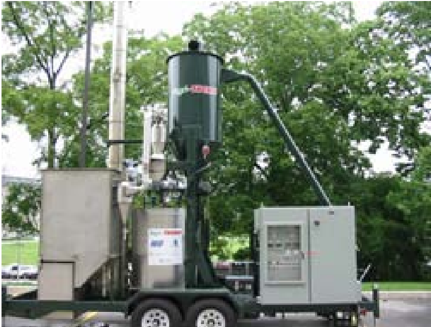
A mobile pyrolysis reactor from Agri-Therm
