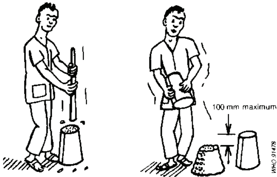
Fig. 7.18. Checking the water content of concrete with a slump cone
