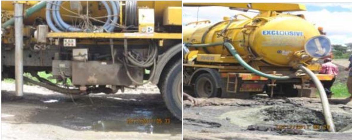
Figure 3-20 : Pump System of an Imported Vehicle
