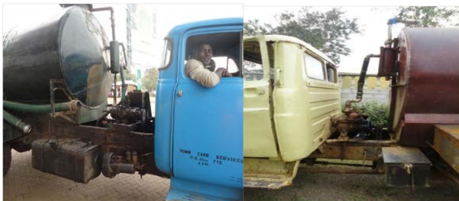
Figure 3-9 : Location of Pumps in Trucks - Kisumu
