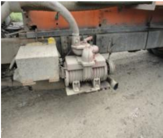
Figure 3-31 : Alternative Pump Technology for Exhauster Trucks
