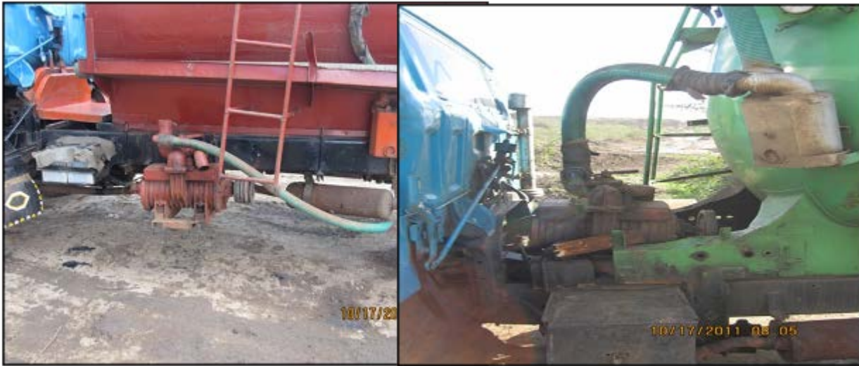
Figure 3-21 : Different Pump Positions for Locally Assembled Trucks
