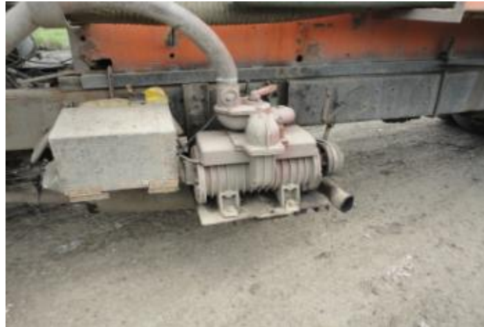
Figure 3-14 : Pump System coupled to Shaft of Truck - Mombasa
